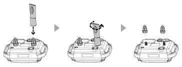
1. Loosen both contact points by rotating the contact point counter-clockwise using the contact point tool.
